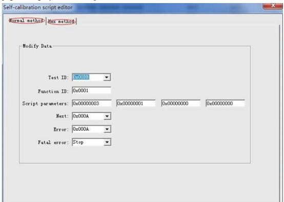
Single process editor is used to fill in the parameters required by individual process. This editor provides two edit modes, of which HEX editing mode can only be used when the user is quite familiar with data structure of individual process.
