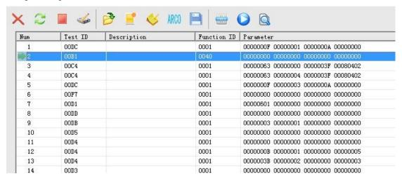
As is shown above, select "Tools -> Self-test series tools -> Offline self-test". After opening, we can see the form of this interface similar to modules list, while here listed test entry information of Module 28. We can perform edit, deletion, adding and other operations to these entries. We can even create a new empty 28 script module, save the modified scripts into file and load edited template of script module for using.
