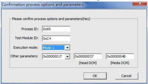
After clicking "->", the process will not be added to the list on the right immediately. We need to adjust and confirm some parameters to make the success rate of test higher. Usually the parameters needed to be paid attention are:
