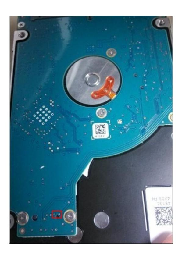
Other laptop HDD short circuit contacts: Appearance of PCB is below:
